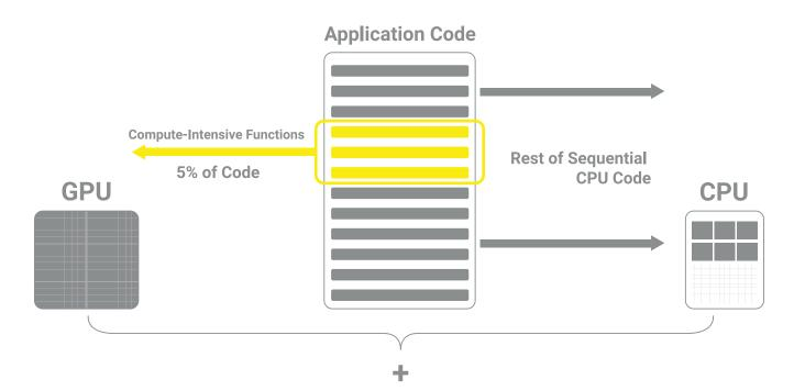
Some processes are inherently sequential and achieve best results with the CPU, and they will always be a part of any complete solution. Many other parallel application processes can benefit from GPU resources. For that reason, using CPUs and GPUs in combination takes advantage of the best of both technologies, tapping the impressive sequential processing power of the latest generation of CPU with the exponential capacity for parallel processing offered by top-performing GPUs.
